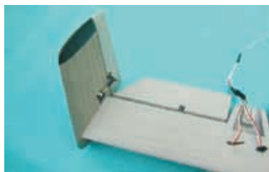
5.11 Connect the horizontal tail wing and vertical tail wing together as shown.
