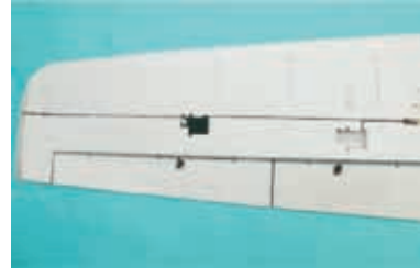
6.4 Install the aileron servo in place.
