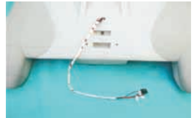
3.12 Bind the wires together.
