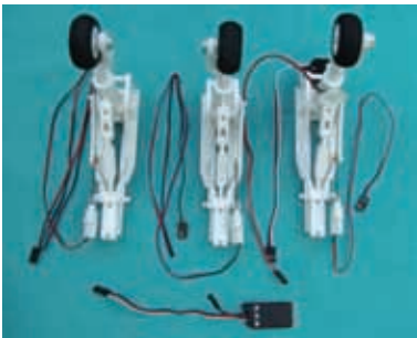
3.1 Retractable landing gears are as shown.
