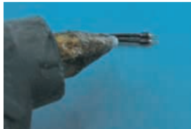
11.8 Apply some foam safe hot glue on the wire.
