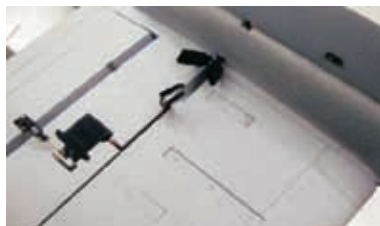
16.5 Install the wires of aileron servo and flap servo as shown.
