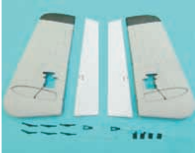
5.1 Need the following parts to assemble the vertical tail wing: 2pcs 33mm long push rods, 2pcs buckle, 4pcs 1.7*10mm screws and 6pcs hinges.
