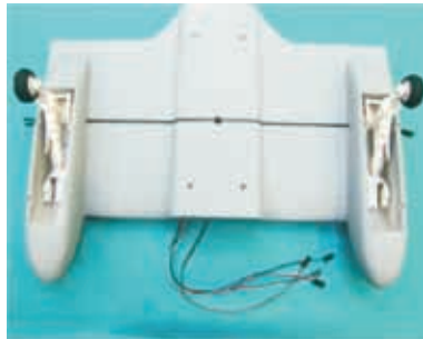
3.11 Assembly for back landing gear is finished.
