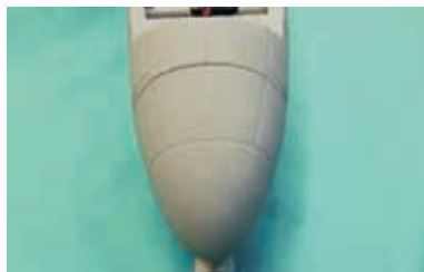
14.1 Glue the front nose on fuselage.
