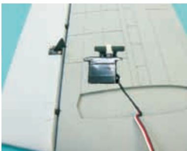
5.7 Apply glue on servos and insert the servos into the slot.
