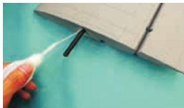
16.2 Insert the pipes into the holes and secure the pipes with glue.
