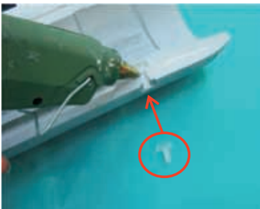
1.7 Insert the holders in slots and fill the space with foam safe hot glue.
