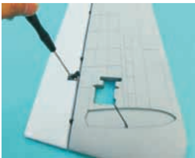
5.4 Install the horns on rudder.
