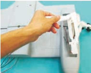
3.10 Assembly for back landing gear is same as front landing gear.
