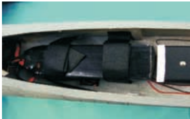
15.1 Install the battery as shown. (Do NOT connect battery at this time)
