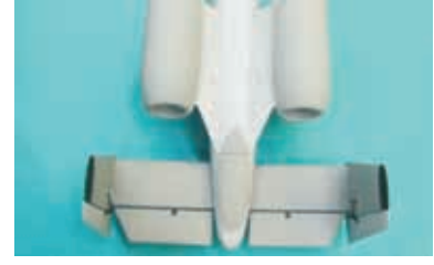
8.2 Install the ducted fan engine on the fuselage.
