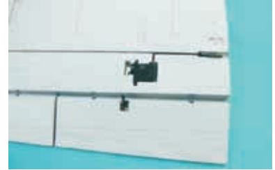
6.5 Install the flap servo in place.
