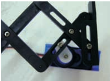
11.16 Install the cockpit ejection system and servo arm together.
