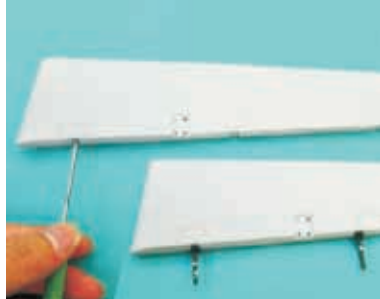
5.2 Punch a hole in the slot. Then spread some glue on the hinges and insert the hinges into the holes.
