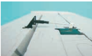
6.6 Install the aileron push rod as shown.
