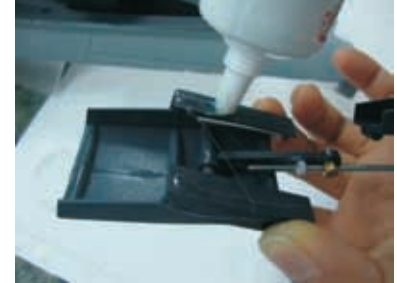
11.3 Apply some glue on the bottom and assemble the lift system as shown.
