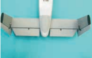
7.4 Install the tail wing on fuselage.
