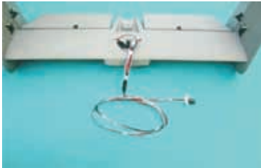
6.1 Bind all the wires together.
