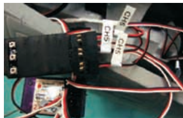
14.2 Install landing gear controller as shown (Only Positive and Negative servo wires are to be connected)
