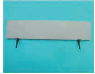
3.6 Spread some glue on the hinges, and then insert the hinges into the holes.
