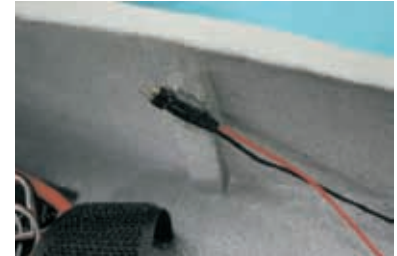
11.9 Secure the wire under the canopy as shown above.
