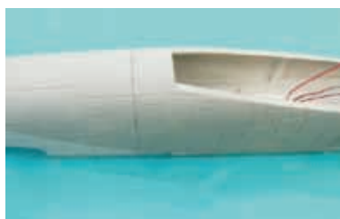
7.2 Assemble the front and back fuselages together.
