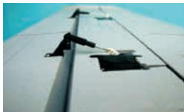
6.7 Install the flap servo push rod as shown.
