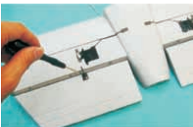
4.4 Install the horns on elevator.
