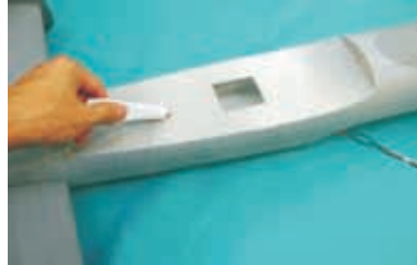
8.1 Apply glue on the contact surface.
