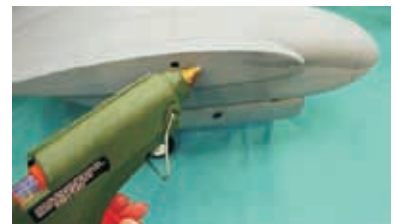
16.3 Apply foam safe hot glue on contact surface shown above.
