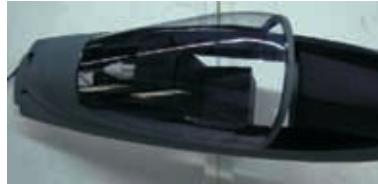
11.5 Glue the back canopy on the lift system.
