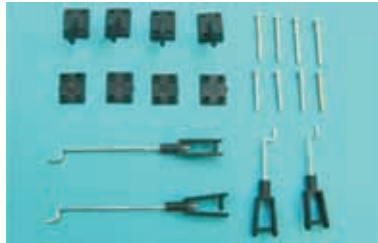
6.2 Need the following parts: 2pcs 39mm aileron push rods, 2pcs 23mm flap push rod, 4pcs buckle, 4pcs 1.7*18mm screws and 4pcs 1.7*15mm screws.
