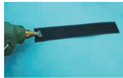
10.3 Spread foam safe hot glue on the belt.
