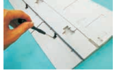
6.3 Install the horns in place .
