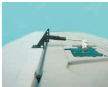
5.8 Install the push rods as shown.
