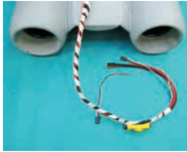
1.14 Bind all the wires together.
