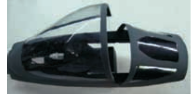
11.6 Front canopy is assembled as shown.
